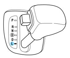
The automatic transaxle will shift into the proper gear to ascend any grade without any need to shift to L (Low).
